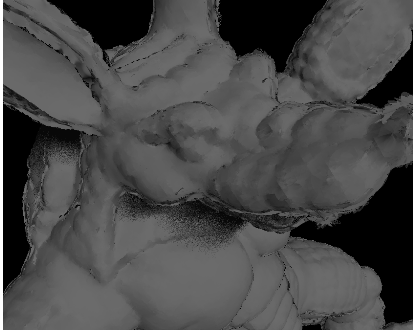
Figure 13: Rendering results for the Armadillo (173k points) using runtime normal estimation. The disc size is doubled in comparison to the approaches using normals. This is required generate enough intersections for the normal estimation. The increased disc size results in less quality on fine structure.
