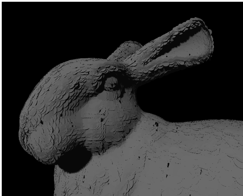
Figure 4: Bunny [1] (36k Points) rendered using discs. Shadow effects between neighboring discs can be seen.
