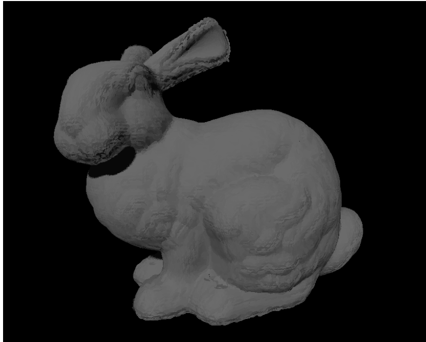
Figure 5: Bunny [1] (36k Points) rendered using discs. Using a minimum intersection distance to avoid shadow artifacts. The boundaries of the discs can be seen slightly.
